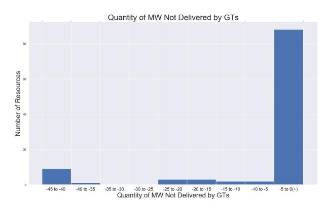
This graph shows the distribution of the quantity of MW not delivered (total energy expected minus total energy provided) for 10-Minute GTs when asked to convert reserves to energy when an RPU was activated in real time
